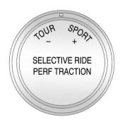
To select a mode while in Performance Traction Management, turn the knob located on the console.
